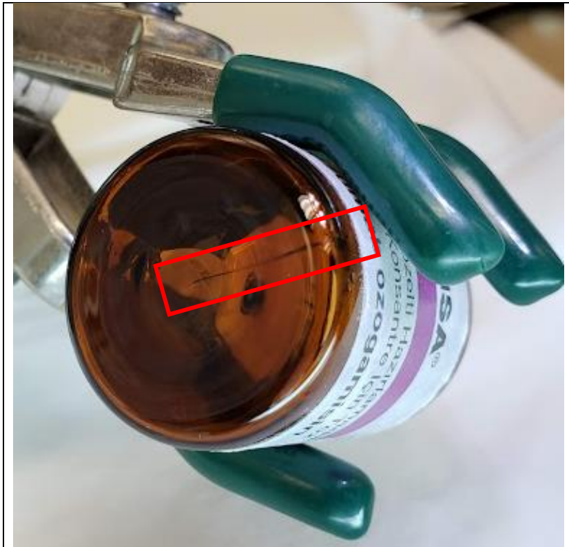
Photo 3 – Vial with Crack on Bottom (highlighted in the red outline)
