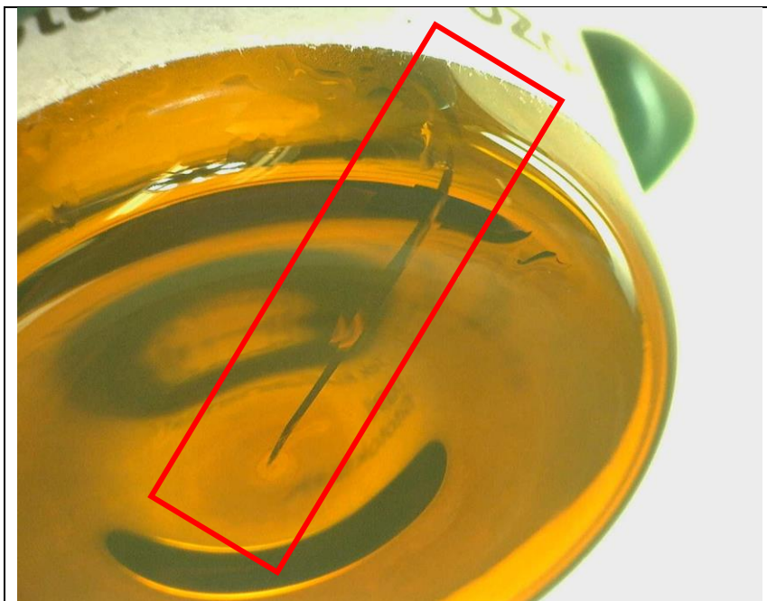
Photo 4 – Vial with Crack on Bottom and Heal (highlighted in the red outline)
